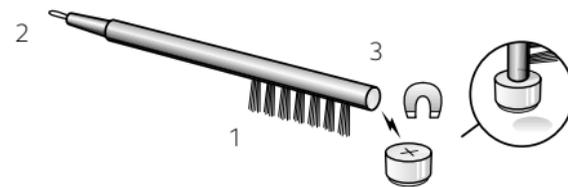
1. Brush - cleaning: Use the brush on all surfaces and orifices
