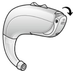
Open the battery door to the OFF position.
