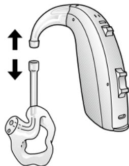
*Pull the earmould and device apart.*
