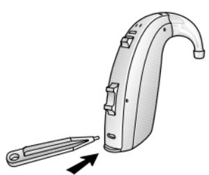
Insert tool straight into battery door lock.
