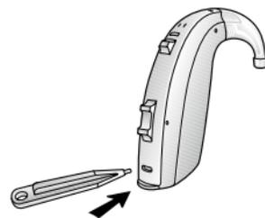
Insert tool straight into battery door lock.
