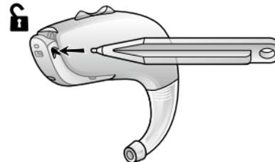
Open the battery door to the OFF position. From the right side, push the slider to the left.
