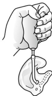
*Use air bulb to remove residual water.*
