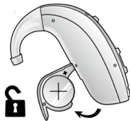
Open the battery door completely to replace the battery.
