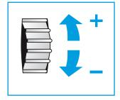
volume setting for you. Please note the setting of that particular level. To increase the volume with the instrument fit to your ear, turn the volume control wheel up. To reduce the volume, turn the wheel down.
