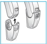
The sound source is connected to your instrument with a cable or a wireless FM system to the audio shoe. The audio shoe will connect with a "click" to the hearing instrument but needs to be switched manually to Direct Audio Input via the programme selector.
