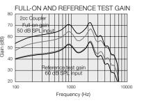
Data in accordance with ANSI S3.22-2009; and IEC 60118-7 ed.2.0 Supply Voltage 1.3 V, 2cc coupler
