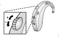
Your hearing care professional may have activated a function in the hearing instrument enabling the instrument to learn how you adjust the volume control in different listening environments. As it learns your volume preferences, the instrument eventually changes the volume for you automatically. This function can be turned off or reset by your hearing care professional.
