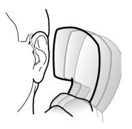
By selecting the optional telecoil programme you can improve understanding of speech when using a hearing instrument compatible telephone. Rather than picking up the sound from the telephone, this programme only picks up the telephone's magnetic signal and converts it to sound. Your hearing care professional can activate the telecoil.
