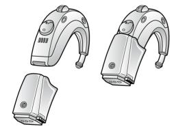
The sound source is connected to your instrument with a cable or a wireless FM system to the audio boot. The audio boot will connect with a "click" to the hearing instrument and switch to Direct Audio Input automatically.
