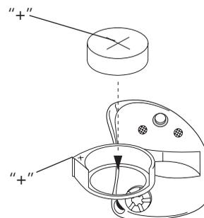
Always use the correct zinc-air battery size for your instrument. Please note that if the battery is weak, the hearing instrument performance will be reduced. Removing the battery when you are not wearing the instrument will help prevent corrosion of the battery contacts and reduce battery consumption.
