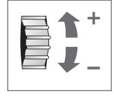
setting for you. Please note the setting of that particular level. To increase the volume with the instrument fit to your ear, turn the volume control wheel up. To reduce the volume, turn the wheel down.
