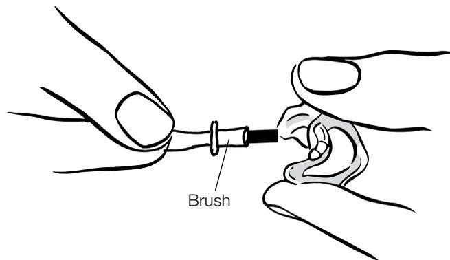
Be sure to thoroughly dry the ear mould and its tubing before connecting it to the hearing instrument. Gently blowing in the tubing will remove dry water trapped inside.
