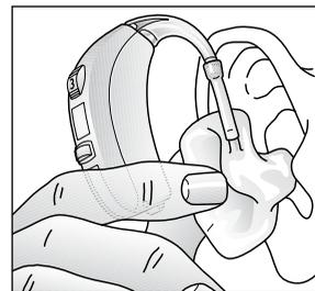
2) Slide the ear mould all the way into your ear with a gentle, twisting movement (insertion will be easier if you gently pull your ear up and back with your other hand)
