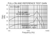
Data in accordance with ANSI S3.22–2003 and IEC 60118-7; Supply Voltage 1.3 V, 2cc coupler
