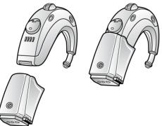
The sound source is connected to your instrument with a cable or a wireless FM system to the audio boot. The audio boot will connect with a "click" to the hearing instrument and switch to Direct Audio Input automatically.
