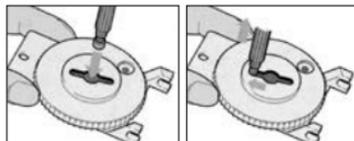
in the wax guard kit by pressing it into the center, sliding it to one end of the slot, and pull until the filter is discarded.
