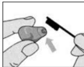
2. Insert the threaded end of the wax guard tool into the used wax guard, and rotate clockwise.
