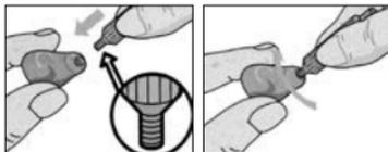
3. Gently pull until the used guard is removed.
