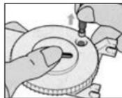
7. Press the new guard to the canal tip of the hearing aid. Move the tool gently side to side and pull it away from the hearing aid.
