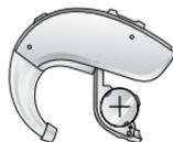
4. Gently close the battery door. If it doesn't close easily, check to see if the battery is upside down.
