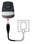
When fully charged and still connected to the charger, the LED will turn solid green interrupted by a red blink every 2 seconds.
