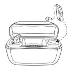
If there is a sports lock attached to your receiver, be careful when placing the receiver into the charging bay.
