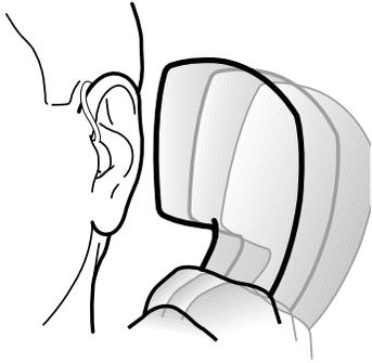
By selecting the optional telecoil programme you can improve understanding of speech when using a hearing instrument compatible telephone. Rather than picking up the sound from the telephone, this programme only picks up the telephone's magnetic signal and converts it to sound. Your hearing care professional can activate the telecoil.
