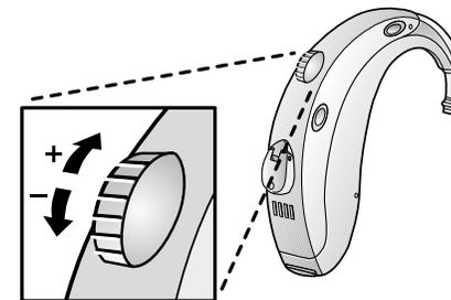
Your hearing care professional may have activated a function in the hearing instrument enabling the instrument to learn how you adjust the volume control in different listening environments. As it learns your volume preferences, the instrument eventually changes the volume for you automatically. This function can be turned off or reset by your hearing care professional.
