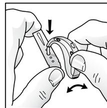
Place the hook on one filter and push gently. Rock the hook back and forth until the filter is released
