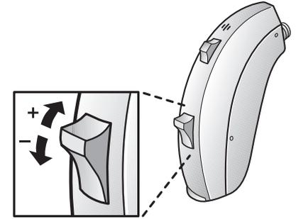
Your hearing care professional may have activated a function in the hearing instrument enabling the instrument to learn how you adjust the volume control in different listening environments. As it learns your volume preferences, the instrument eventually changes the volume for you automatically. This function can be turned off or reset by your hearing care professional.
