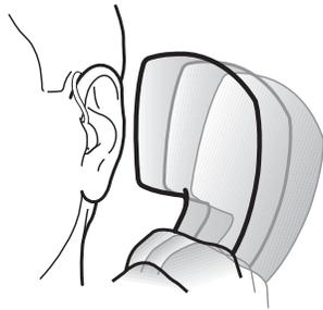
When using the telecoil programme, the receiver of the telephone should be held as shown in the drawing. You may need to move the handset around slightly to find the best reception.
