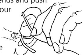
3. Position the Sports Lock into the indentation above the earlobe. If the device whistles, the most likely reason is that the dome is not placed correctly in the ear canal or build-up of earwax in the ear canal. It is also possible that the instrument settings are not optimal. If you have ruled out other reasons for the instrument squealing, it is recommended to contact your hearing care professional.
