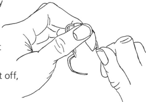
To turn the instrument off, grasp the battery compartment door with your fingernail and gently pull. The power will switch off at the point where you can feel a small click. Whenever you are not wearing the instrument, remember to turn it off to reduce battery consumption. If you run your ReSound Pulse with rechargeable batteries the charger opens the battery compartment door automatically when inserting.
