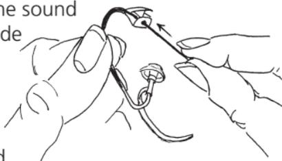
tube attaches to the instrument and pushed all the way through the sound tube and out through the dome. It is not recommended to submerge or rinse the sound tube and dome with water, as there is a risk that a water drop may become lodged in the sound tube. If this should occur, it will prevent sound coming through the sound tube, and may be harmful for the instrument’s electronics.
