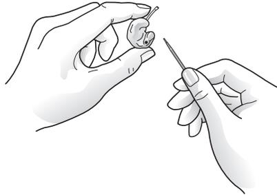
The tubing connecting the earmould to the hearing instrument should be changed if it becomes stiff or brittle. Contact your hearing care professional to change the tubing when needed.
