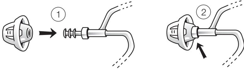
1. Push the dome over the grooves on the tube to mount it (1) + (2).
