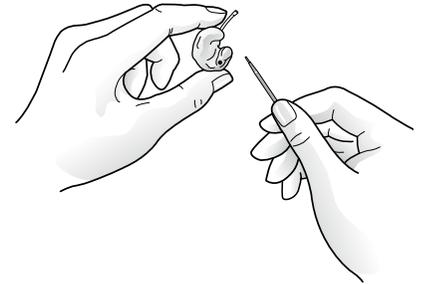
The tubing connecting the earmould to the hearing instrument should be changed if it becomes stiff or brittle. Contact your hearing care professional to change the tubing when needed.
