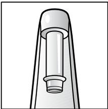
Your ReSound Ziga hearing instrument is equipped with a filter. This filter is located at the top of the sound outlet and prevents moisture and debris from getting into the hearing instrument. If the hearing instrument seems to have lost power and changing the battery does not help, the filter may be blocked, and needs to be changed. See instructions below:
